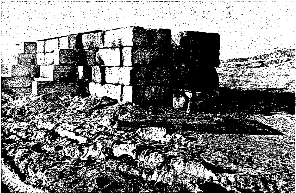
Fig 14. Firing 3. Showing roof plate and half Pendine block thrown off. (Neg Ref 6390).
